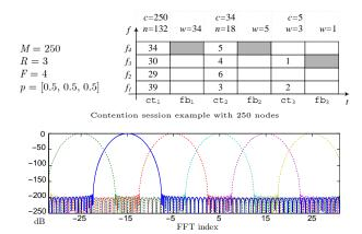
*Time-Frequency contention.* A fast-converging round-based algorithm where nodes are eliminated by peers or *referees* by randomly bursting and sensing short (5  $\mu$ s), unmodulated and "*cached*" OFDM subcarriers.
