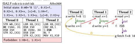
Here the IC gets broadcast to all threads [9, B2.2.5p3], and so the fact that it happens on a different thread to the DC does not affect the outcome. Similarly, if the DC were to happen on another thread first (to get the test MP.RF+[dc]-ic+ctrl-isb, not shown), then it would have the effect of ensuring consistency globally, for all threads.
