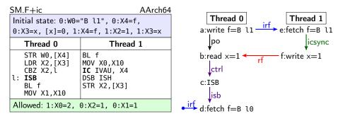
new value and performs just an IC and DSB, before signalling Thread 0 which also fetches f. That IC is not strong enough to ensure that the write is pulled into the instruction cache of Thread 0.
