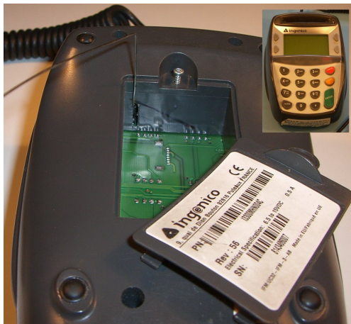
(a) A paperclip is shown inserted through a hole in the Ingenico's concealed compartment wall to intercept the smartcard's data. The front of the PED is shown on the top right.
