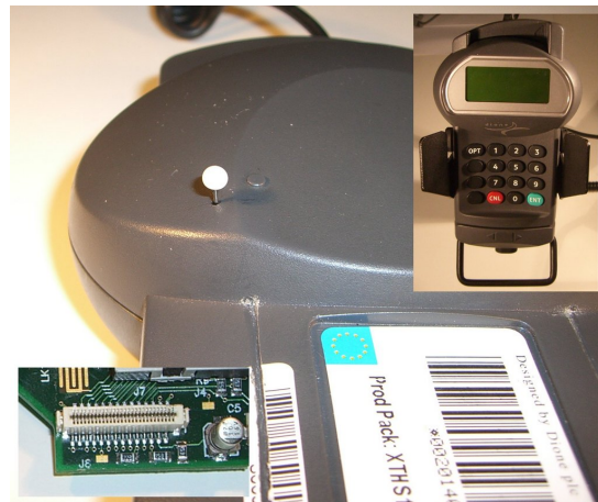
(b) A needle is shown inserted through the rear of the Dione PED for data interception, attaching to a ribbon cable connector shown on the bottom left; a mounted PED is in the top right.
