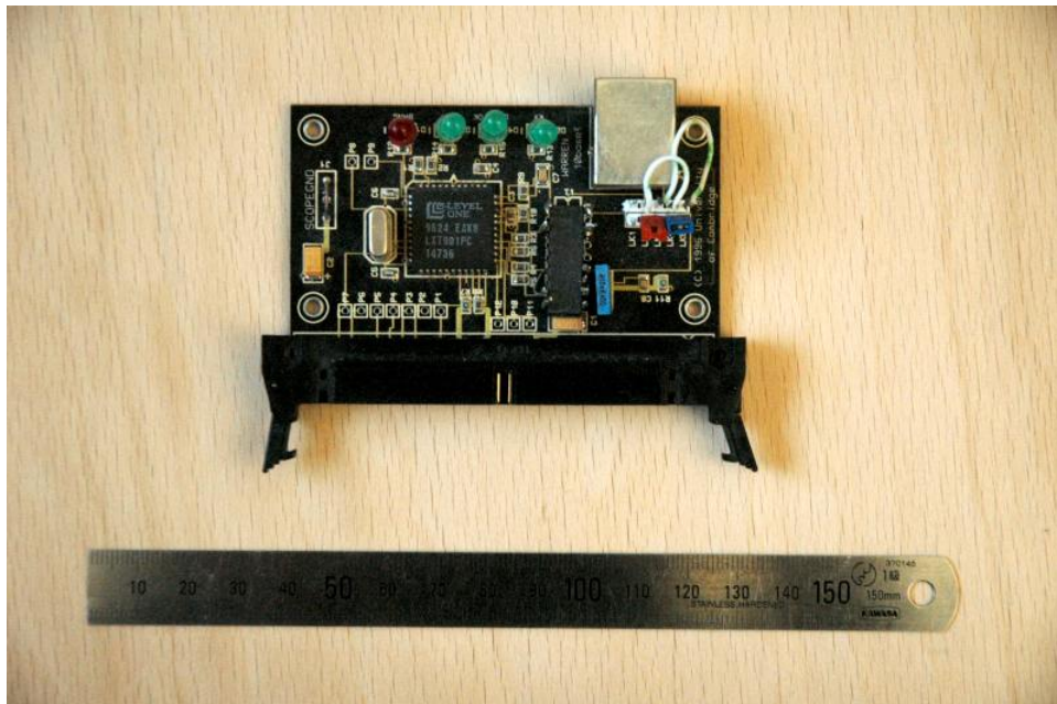
Figure 4.3: Warren PCB showing Intel LXT901
