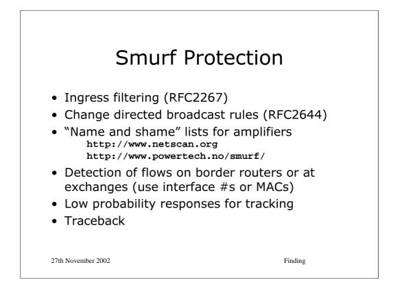
★ If systems didn't let forged packets out onto the Net then all would be wonderful (see RFC2267). Unfortunately it is seldom simple for complex networks to install suitable filtering.
