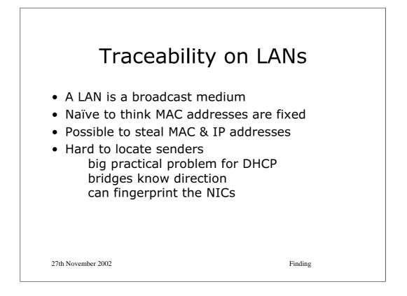
★ Ethernet LANs are a broadcast medium (using CSMA/CD to share the channel capacity). Nodes are identified by a Media Access Control (MAC) addresses which are supposed to be unique [the first 24 bits is the Organizationally Unique Identifier (OUI) assigned to a vendor and the second 24 bits is a serial number].
