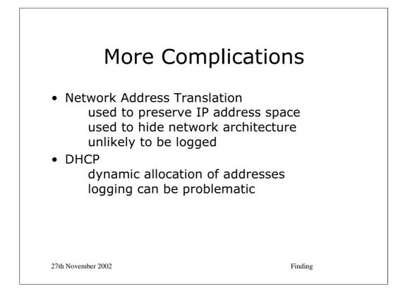
★ Network Address Translation (NAT) is widely used to conserve address space, to allow the operation of several machines on a single dial-up connection and for security reasons by ensuring that machines are not visible to the open Internet. The IP address recorded at a remote site is likely to be the address of the kit doing the NAT. Mapping this to a particular machine "behind the NAT" is unlikely to be possible since it is rare to record NAT assignments in logs.
