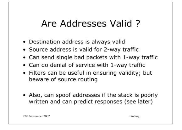
★ If you are not interested in getting packets back from a remote machine then the validity of the source address is irrelevant. If you wish to avoid being traced then you might set an invalid address. There are a number of attacks that are possible with 1-way traffic such as denial of service attacks and the sending of malformed packets that crash the remote system.
