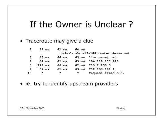
★ *traceroute* works by sending ICMP echo requests (or sometimes UDP packets) with a small "hop count". As the packets traverse each machine along the way to their destination the "hop count" is progressively reduced. When it expires, an ICMP "hop count exceeded" packet will be generated and sent back to the source machine. By progressively increasing the hop count it is possible to map the outgoing path.
