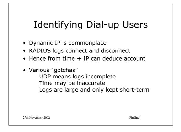
★ Dial-up connections to the Internet are usually given a "dynamic IP address". ie: the IP address depends upon the modem port used or is taken from a small pool of addresses rather than being dependent upon the account being used for connection.
