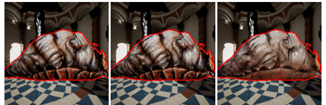
Figure 2: Example of one scene from the dataset with 3 texture resolution variants of albedo map: highest resolution (left), medium resolution (middle), and lowest resolution (right). The target object in the scene has a red outline to prevent it from blending with the background.
