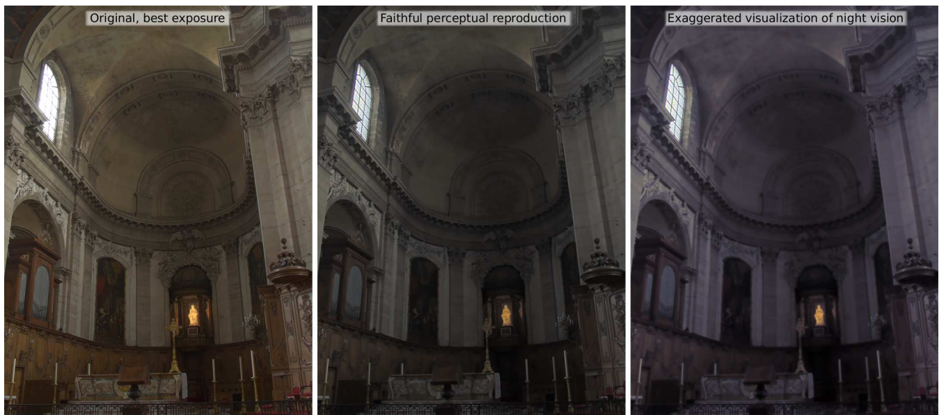
Figure 13: Best exposure from a scene-referred HDR image (left) compared with a faithful simulation of night vision (center) and exaggerated rendering for a more dramatic effect (right). Compare the differences in the visibility of details and color.
