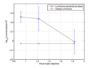
**Figure 9:** The results of the experiment, shown as blue lines with error bars, indicate the highest luminance the participants could not distinguish from the lowest luminance we could achieve in our laboratory conditions  $(0.024 \text{ cd/m}^2)$ . The red markers indicate the measured black level of our display for the same pattern as used in the experiment but with the ND filter removed.
