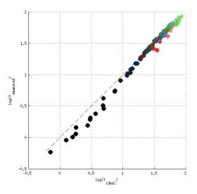
**Figure 4:** The expected and measured luminance of our display in  $\log_{10}(cd/m^2)$ .
