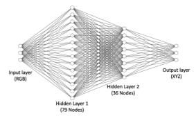
Figure 3. The demonstrative architecture of the neural network. Input and output layers consist of 3 nodes which are RGB and XYZ respectively. In between, there are 2 hidden layers formed by 79 and 36 nodes.
