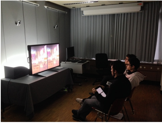
Fig. 2. Three observers assessing a test image relative to a reference image shown on the SIM2 HDR monitor, in viewing conditions conforming to the ITU-R BT.500-13 recommendation.
