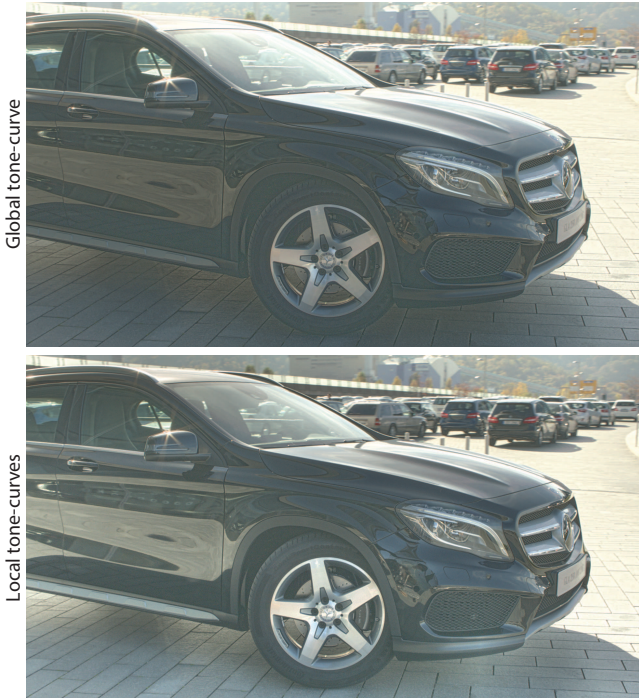
Figure 5: Tone-mapping using global (top) or local (bottom) tone-curves. The image was generated assuming high ambient light viewing (low contrast) to better show contrast reduction. Note that other components of the operator, such as local contrast, were disabled for this example.
