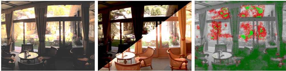
Figure 1: Quality assessment of an LDR image (left), generated by tone-mapping the reference HDR (center) using Pattanaik’s tone-mapping operator. Our metric detects loss of visible contrast (green) and contrast reversal (red), visualized as an in-context distortion map (right).
