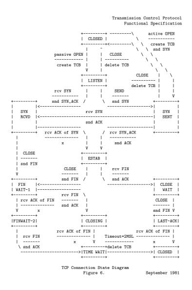
Figure 16: The RFC793 TCP state diagram
