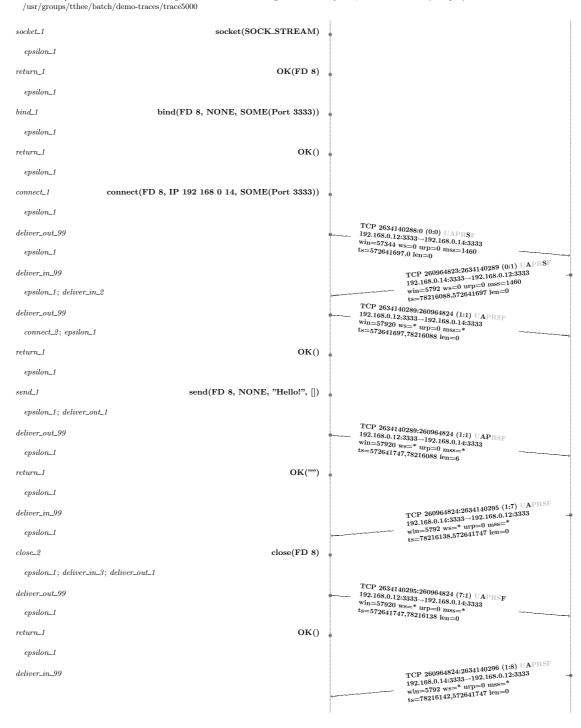
Figure 7: Sample checked TCP trace, with rule firings – connect() end
