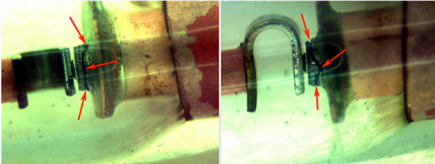
Figure 1. Two views (90 degrees apart) of a fissure that appears to go through the silicon dice - Red arrows.
