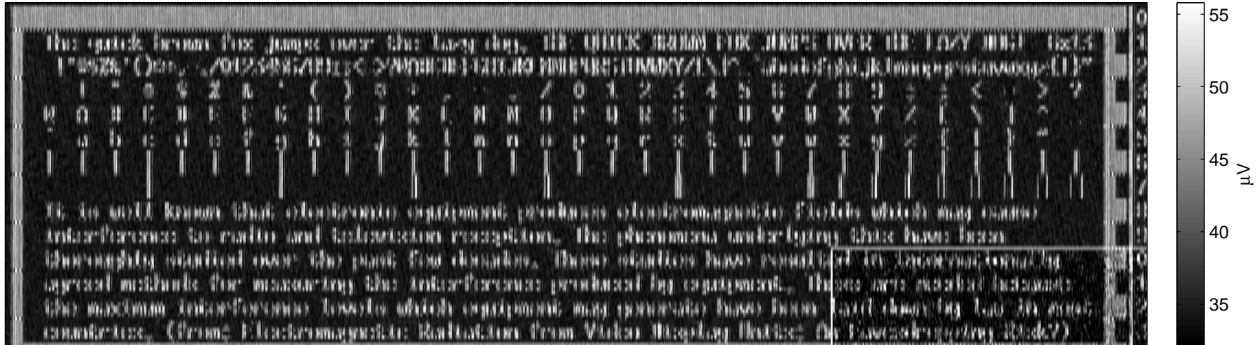
480 MHz center frequency, 50 MHz bandwidth, 256 (16) frames averaged, 3 m distance
