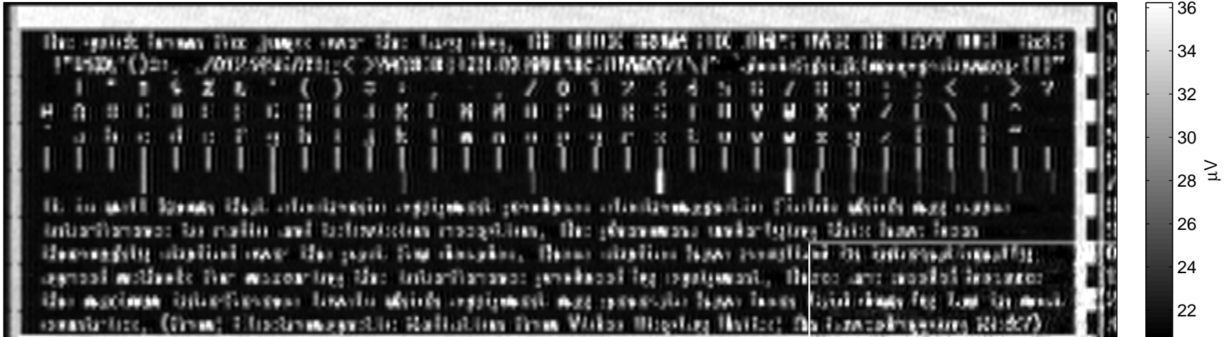
292 MHz center frequency, 20 MHz bandwidth, 256 (16) frames averaged, 3 m distance
