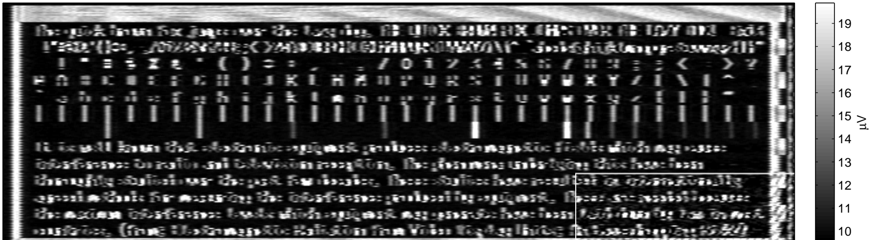
292 MHz center frequency, 10 MHz bandwidth, 256 (16) frames averaged, 3 m distance
