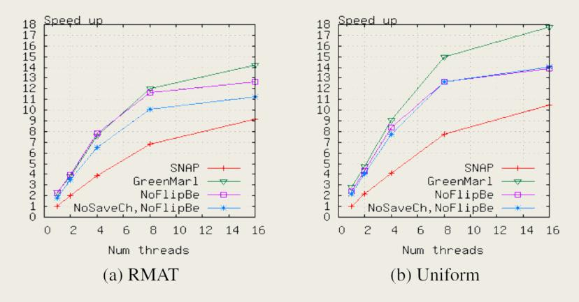
**Figure.** Speed-up of Betweenness Centrality. Speed-up is over the SNAP library [9] version running on a single-thread. NoFlipBE and NoSaveCh means disabling the Flipping Edges (Section 3.3 Architecture Independent Optimizations) and Saving BFS Children (Section 3.5 Code Generation) optimizations respectively.
