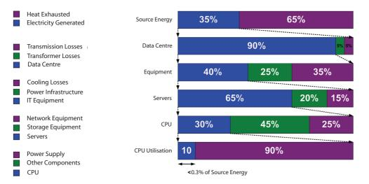
Figure 2: Diagram showing where energy is lost between source and processor in a 2007 vintage data centre (image courtesy of Liam Newcombe)
