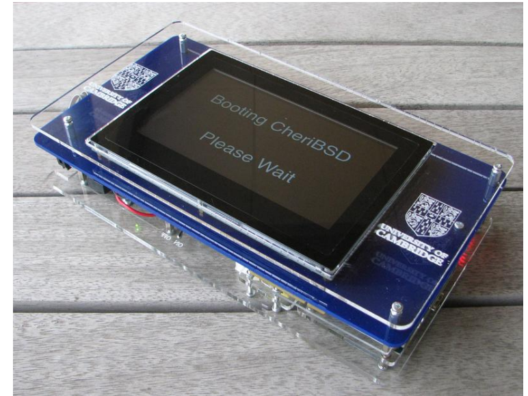
DE4 prototype tablet computer running CHERI, origin unknown, https://www.cl.cam.ac.uk/research/comparch/opensource/de4tablet/tablet-booting-cheri.jpg
