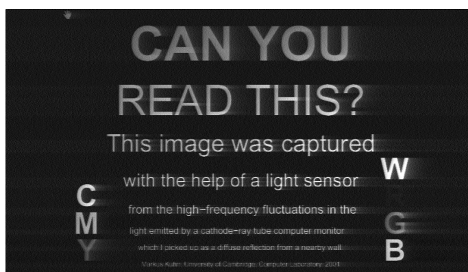
eavesdropping result after deconvolution
