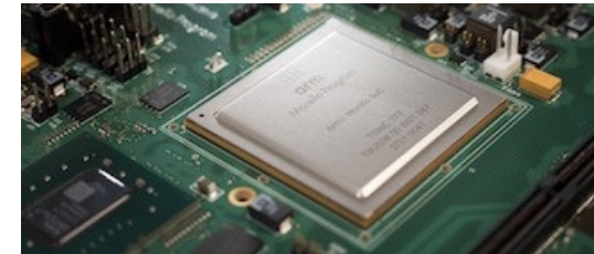
High-performance Arm Morello chip able to run a full CHERI software stack, Cambridge, 2022
