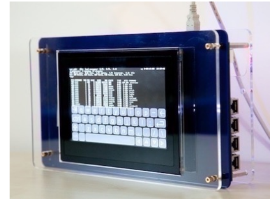
An early experimental FPGA-based CHERI tablet prototype running the CheriBSD operating system and applications, Cambridge, 2013.
