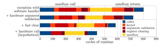
Figure 2: Total cycle count, spanning userspace and kernel, for a zero-byte memcpy in a sandbox
